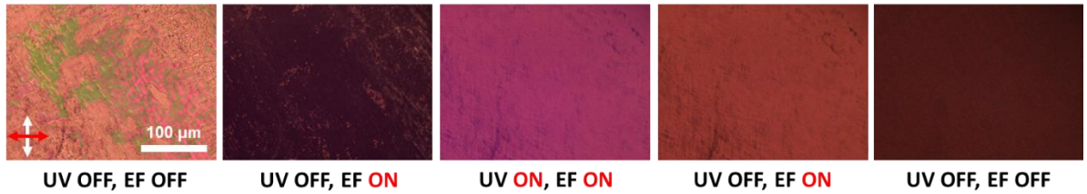
Fig. S2. Polarizing optical microscopy (POM) images of the polymerized sample with crossed polarizers during polymerization at T = 45 \text{ }^{\circ}\text{C} . The cell thickness is d = 20 \mu\text{m} .
